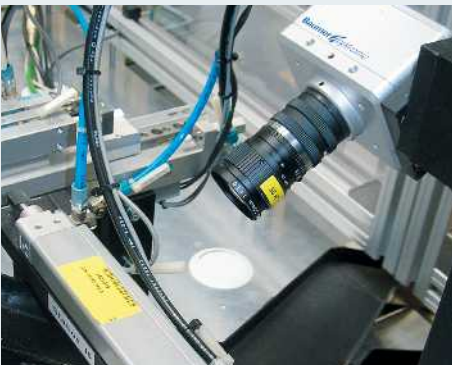
Quality inspection using optical camera systems
