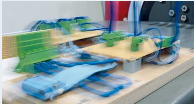
Mechanical load tests through vibration tests
