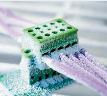
Durability test under extreme climatic conditions
